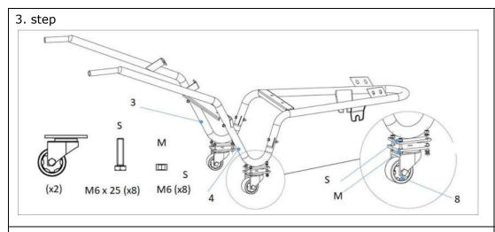
Assemble one support wheel (8) to each handle (3,4) using screws (S) and nut (M).
