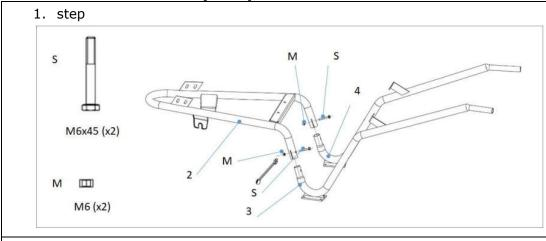
Assemble the left (3) and right handle (4) to the frame (2) using one screw (S) and nut (M) each.
