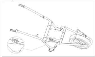
Assemble the 3 wires to the battery box.
