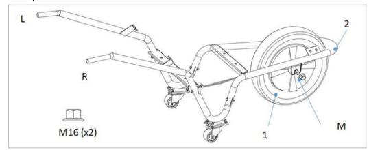
Mount the motor wheel (1) with 2 nuts (M) on the support frame (2).
