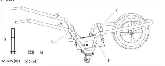
Assemble the battery box (6) to the frame (2) and support (5) using screws (S) and nut (M).
